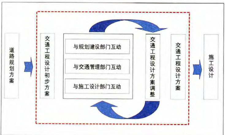
图12 道路规划设计建设总体协调 Fig.12 Overall coordination among road planning, design and construction
